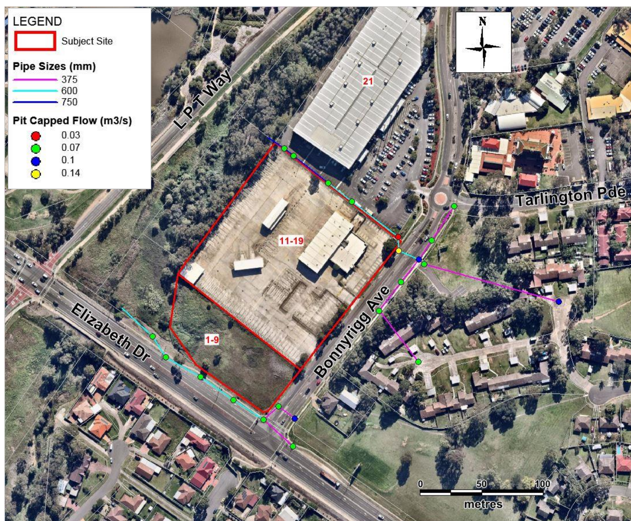
Figure A3 – Modelled Street Drainage Pits and Pipes
